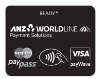
An asterisk (\*) is displayed when the terminal has stored Electronic Fallback (EFB) transactions.
