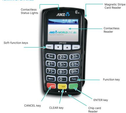
The ANZ POS Plus 2 terminal incorporates a large colour graphic screen, 18 function keys, a Magnetic Stripe card Reader, a Chip card Reader and a built-in Contactless Reader.
