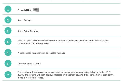
**Note**: If the terminal fails to connect to any of the above communications modes and you wish to have them enabled with Auto-Comms Fallback, please check and ensure the cables are connected securely and re-try.
